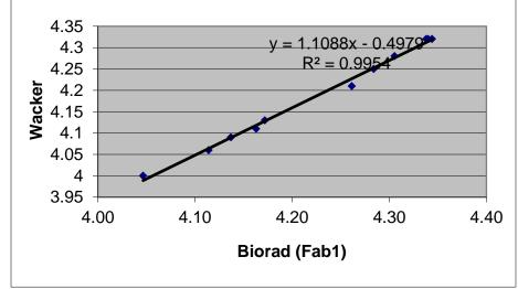
Through the measurement points, a line has been fitted with the following equation Y = 1.1088x - 0.4979
